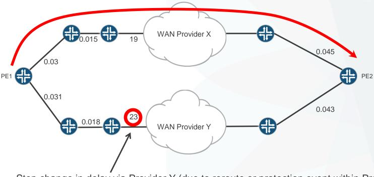
Step change in delay via Provider Y (due to reroute or protection event within Provider Y) Controller reroutes red LSP via Provider X.
